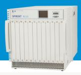
The Spirent dX2 40 GbE and 10 GbE Ethernet test module series offers high density and flexibility for testing next-generation data center multi-terabit fabrics. With support for Ethernet, VLAN, FCoE, IPv4, IPv6, multi-cast traffic generation, and full mesh RFC 2544 latency analysis on thousands of ports, the dX2 module is the industry's high-density and cost-efficient solution for testing switch fabrics to full capacity.
